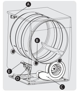
E. **GAS BURNER** (Gas models only.) When the burner is operating, there may be sounds generated as the air flow mixes with the gas flame. This noise is normal and will only occur when the gas is ignited in the combustion tube.
